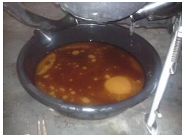
An extreme example of oil contaminating coolant!
