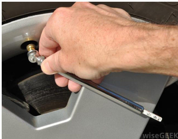
A quick post-race pressure check. Notice the brake rotor and pads visible through the wheel.
