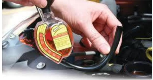
*Be sure to test antifreeze in the radiator, not the overflow*
